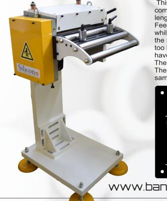
This can be taken into consideration and compensated for by setting a larger feed length on the second feed unit. Feed corrections can also be carried out easily while the press is running. The feed length on the second unit must, however, never be set too long, otherwise this would have a negative influence on the first unit. The result: a diversity of feed lengths. The two operating feed units must be of the same type and their operation synchronized.
